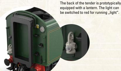
The corridor tender is equipped with a passageway to the train thus allowing crew changes during the train's run. A digitally controlled LED gives a view in the passageway past the coal and water.
