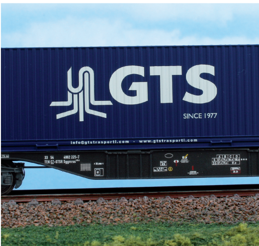
Carro intermodale Tipo Sggmrss '90 "GTS Rail" con casse mobili. Container wagon Type Sggmrss '90 "GTS Rail" with swap bodies. Containerwagen Typ Sggmrss '90 "GTS Rail" mit Wechselpritschen.
