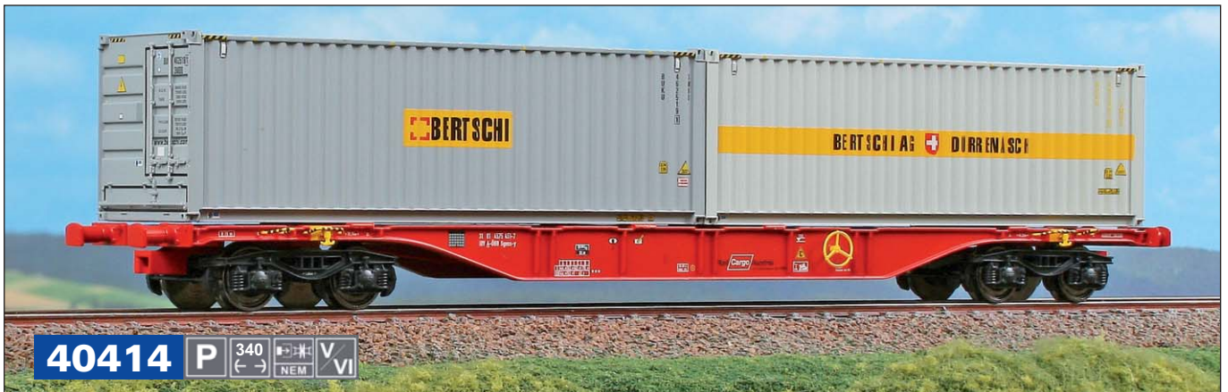
Carro intermodale Tipo Sgnss-y Rail Cargo Austria da 60 piedi caricato con due bulk da 30 piedi "Bertschi". Container wagon Type Sgnss-y '60 Rail Cargo Austria with two "Bertschi" bulk containers. 60-Fuß-Intermodalwagen vom Typ Sgnss-y Rail Cargo Austria, beladen mit zwei 30-Fuß-Bulk "Bertschi".
