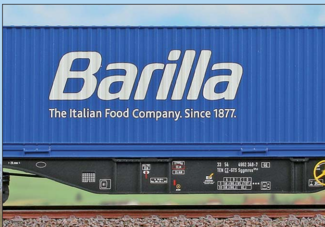
"Il treno della pasta". Carro bi-modulo da 90 piedi GTS con casse mobili "Barilla" e "GTS". "Pasta train". Container wagon Type Sggmrss '90 GTS with "Barilla" and "GTS" containers. "Der Nudel-zug. 90-Fuß-GTS-Bimodul-Wagen mit Barilla- und GTS-Wechselpritschen.
