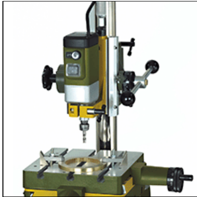
Application on mill/drill unit BFB 2000 and compound table KT 150.
