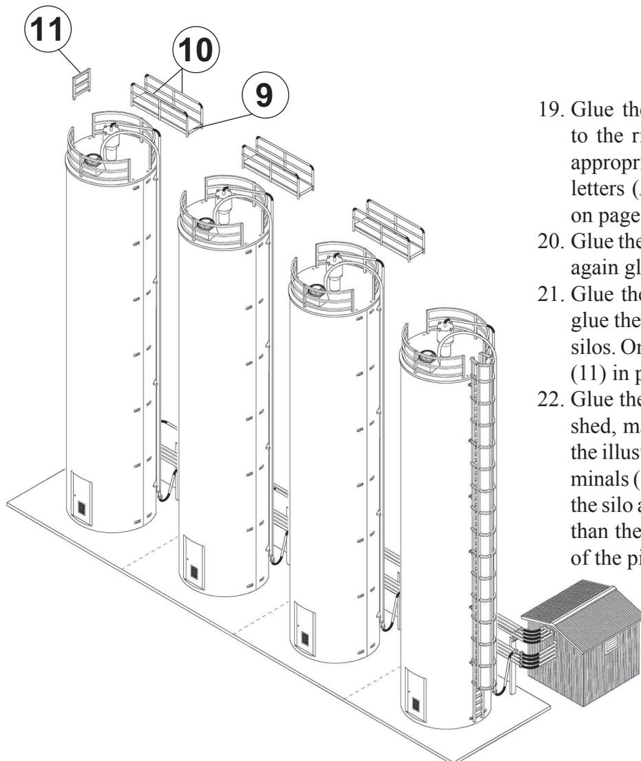
19. Glue the completed silo with the ladder on to the right side of the base (1), gluing the appropriate piping together. Note: Match the letters (A & B) as shown in the illustrations on page 2.
