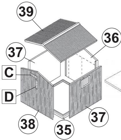
1. Glue the shed walls (36,37,38) together and to the base (35). Then glue the roof (39) on.
