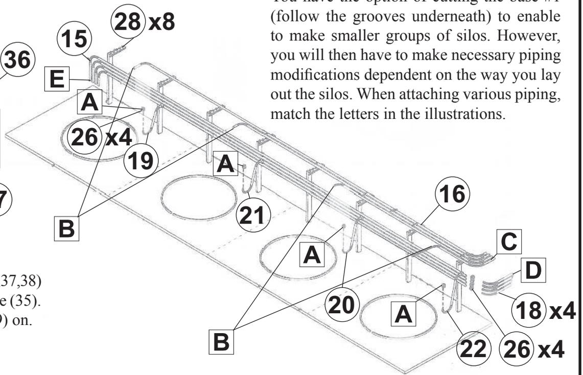
You have the option of cutting the base #1 (follow the grooves underneath) to enable to make smaller groups of silos. However, you will then have to make necessary piping modifications dependent on the way you lay out the silos. When attaching various piping, match the letters in the illustrations.
